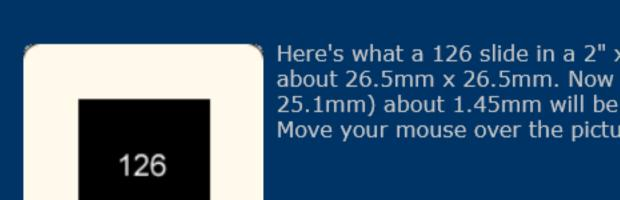
Here's what a 126 slide in a 2" x 2" mount looks like. The viewable area is usually about 26.5mm x 26.5mm. Now due to the aperture of the scanner (36.8mm x 25.1mm) about 1.45mm will be cropped from the top and bottom of these slides. Move your mouse over the picture to see the area that will get cropped out (red).
